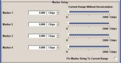
The **Marker Delay** section is where a marker signal delay can be defined, either without restriction or restricted to the dynamic section, i.e., the section in which it is possible to make settings without restarting signal and marker generation.
