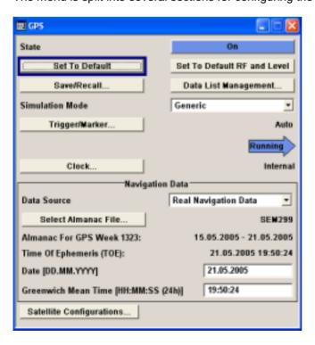
The upper section of the menu is where the GPS digital standard is enabled and the default settings are called.
