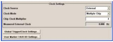
The Clock Settings section is where the clock source is selected and - in the case of an external source - the clock type. The Global Trigger/Clock Settings button leads to a submenu for general trigger and clock settings.
